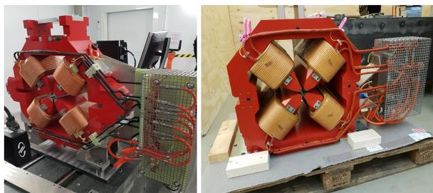
Figure 5: a) MG quadrupole, b) HG quadrupole.
