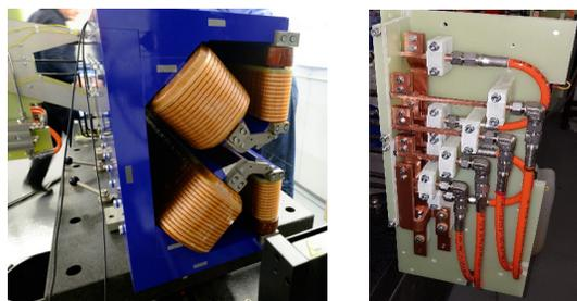
Figure 4: a) Pre-series DQ1 magnet, b) New design of the connections.
