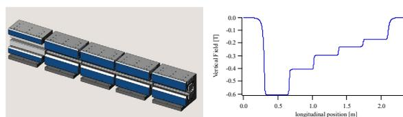
Figure 1: a) DL design with five modules, b) Field versus longitudinal position.
