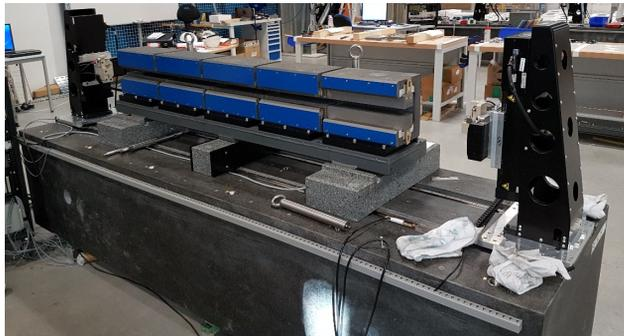
Figure 2: Assembled DL under magnetic measurement.
