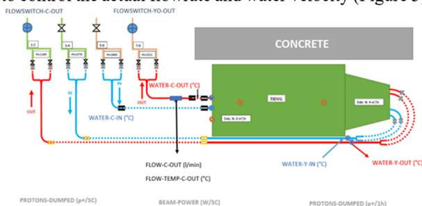
Figure 5. Sensors for the water cooling circuit.
