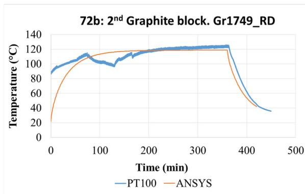
Figure 10: Comparison between simulated and measured temperatures 2<sup>nd</sup> graphite block at steady state for 72-bunch beam.
