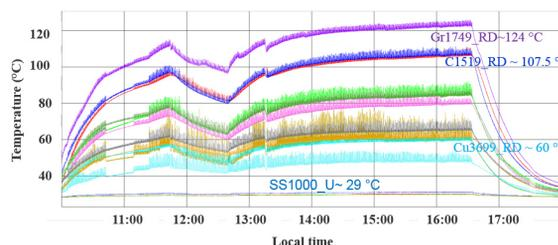
Figure 7: Temperature monitoring for commissioning with 72-bunch beam (steady state reached).
