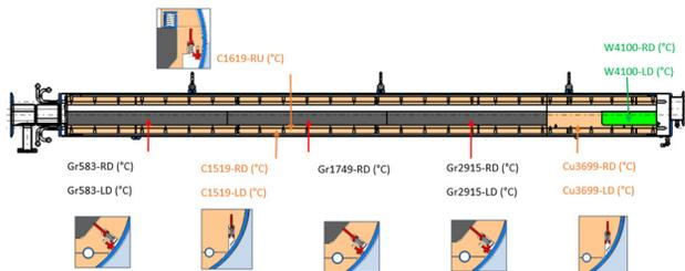
Figure 3. Location of the PT100 temperature gauges in the copper core.
