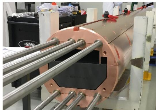
Figure 2: TIDVG#4 core assembly. Upstream face of graphite visible in the lower part.
