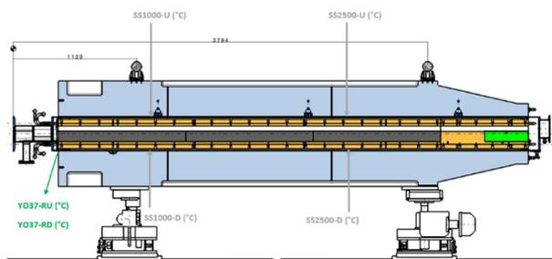
Figure 4. PT100 in the external shielding assembly.
