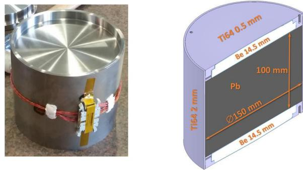
Figure 3. Ti-Pb prototype with beryllium inserts.
