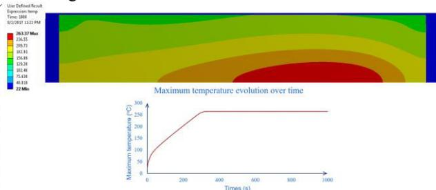
Figure 4. Temperature distribution at steady-state and peak temperature evolution in the accidental scenario (coupled thermo-mechanical analysis).
