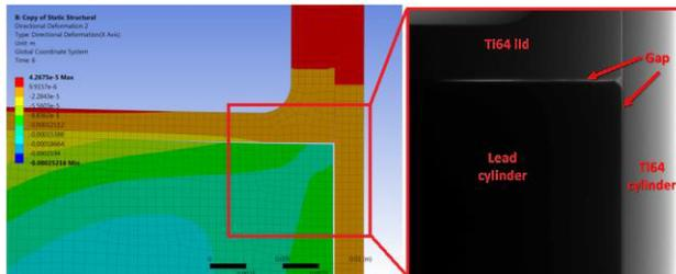
Figure 2. Comparison between simulated Ti-Pb prototype manufacturing process and X-ray inspection results.
