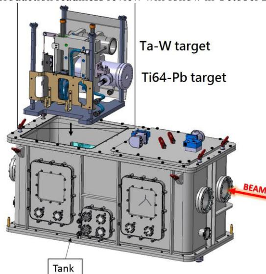
Figure 5.  $n_{\text{TOF}}$  *HiRadMat* experiment tank.
