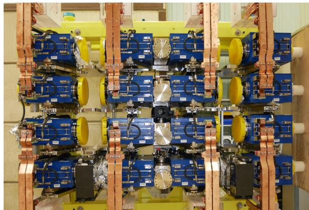
Figure 1: The injection chicane magnets for all 4 booster rings, installed in a mock-up prior to the installation.
