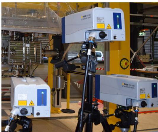
Figure 3: Polytec PSV-500-3D Scanning Vibrometry System.
