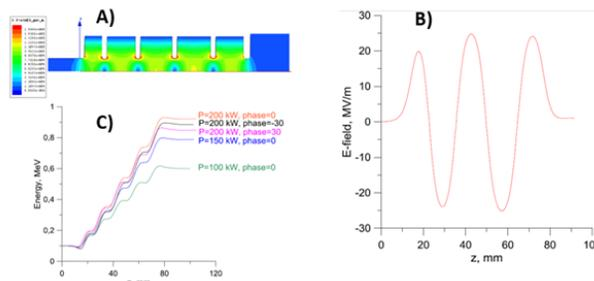
Figure 1: A) z-component of RF electric field. B) field distribution along z. C) energy gain simulations for various input power.
