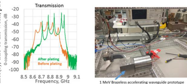
Figure 5: Left: Transmission (S21) measurement before and after plating. Right: Network analyzer measurement of the structure before plating
