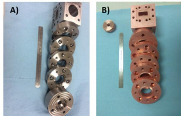
Figure 4: Brazeless assembly manufacturing. A) Stainless steel parts. B) Copper plated parts
