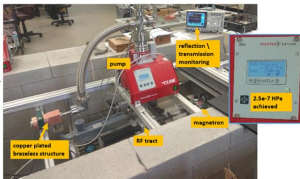
Figure 6: High power test setup with key components identified.
