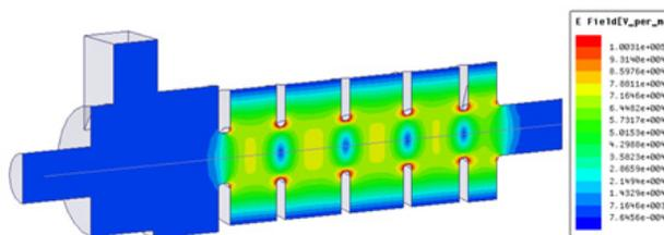
Figure 2: Simulation of coupler and structure (Ez-field).
