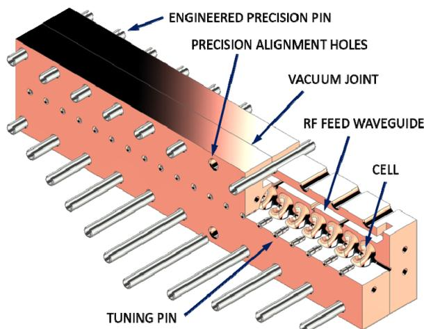
Figure 1: Cut-away view of split section accelerating structure showing the precision alignment features.
