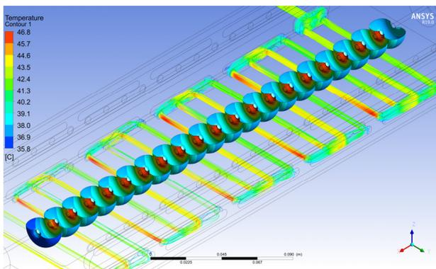
Figure 7: Temperature ( $^{\circ}\text{C}$ ) of the accelerating cells with  $30^{\circ}\text{C}$  coolant inlet temperature. Maximum average temperature is  $46.8^{\circ}\text{C}$  and maximum pulsed temperature is  $49.3^{\circ}\text{C}$ . Streamlines show the relative coolant velocity in the fluid cooling channels.
