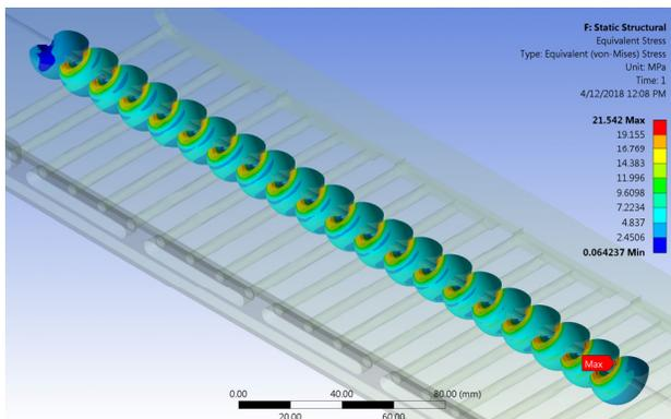
Figure 8: Von-Mises Stress (MPa) on the cell walls with 2.5 kW average power loading. Maximum stress is 21.5 MPa.
