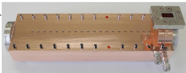
Figure 4: 11.4 GHz brazed 20 cell accelerating structure.
