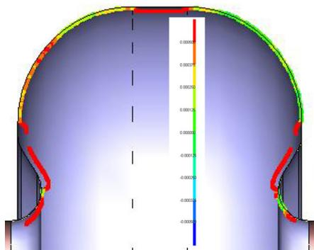
Figure 3: Scanning CMM inspection contour of a sample accelerating cell with deviation shown in inches. The maximum deviation is  $7\ \mu\text{m}$ .
