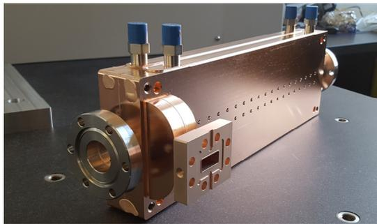
Figure 6: 9.3 GHz X-band brazed accelerating structure.
