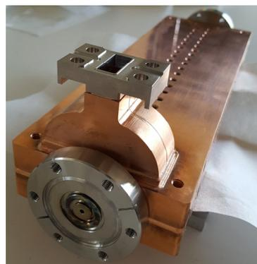
Figure 5: 11.4 GHz electron beam welded accelerating structure with 20 cells fabricated in hard copper alloy.
