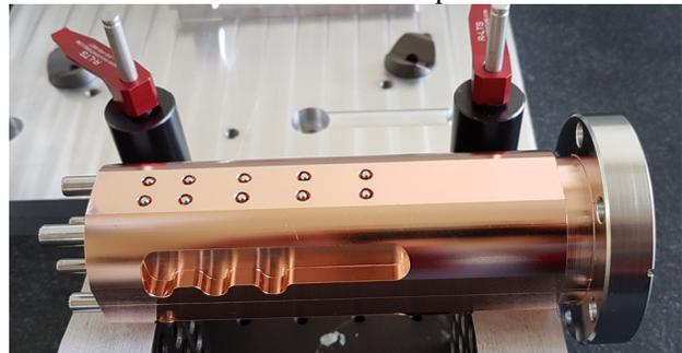
Figure 9: 9.3 GHz RF gun 4.5 cell structure.
