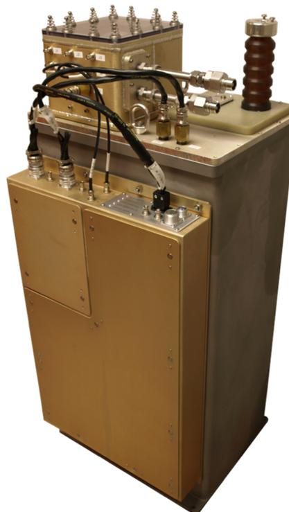
Figure 1: DTI solid-state replacement for the L-4888 thyristor used at SLAC. The switch, which operates at 48 kV and 6.3 kA, fits in the same location as the legacy thyristor assembly.
