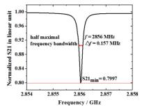
Figure 3: The simulated S21 of the pulse compressor in CST FDS.
