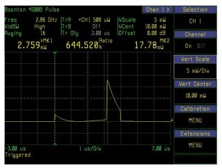
Figure 6: The output pulse waveform of the spherical cavity pulse compressor.
