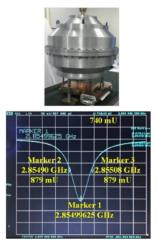
Figure 5: Photo of the fabricated prototype and the tested S21 curve from VNA.
