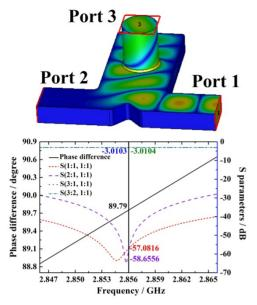
Figure 1: The simulated electrical field distribution and the S parameters of the pulse compressor.
