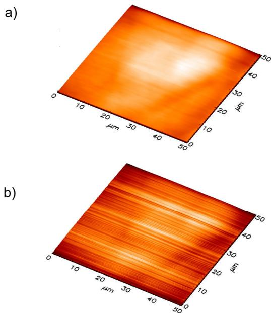
Figure 6: AFM micrographs of Nb surface at initial state (a) and after Ar<sup>+</sup> ion irradiation at 5 keV for 20 min (b).
