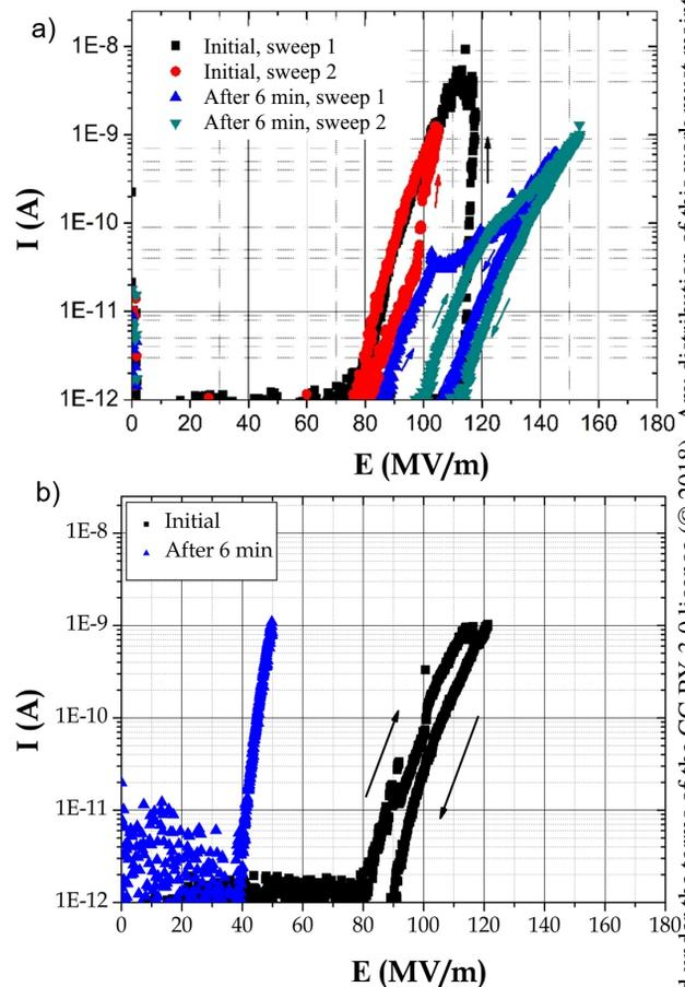
Figure 5: I-E characteristics of emitters before and after the ion irradiation: deactivation (a) and sharpening effects (b) could be observed.
