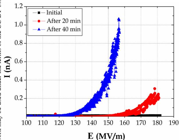
Figure 7: I-E characteristic of an emitter before and after the ion irradiation.
