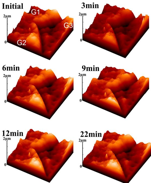
Figure 4: AFM micrographs ( $50 \times 50 \mu\text{m}^2$ ) of the polycrystalline Cu surface before and after 5 keV  $\text{Ar}^+$  ion irradiation for 3, 6, 9, 12 and 22 min. Three different grains (G1-G3) are indicated.
