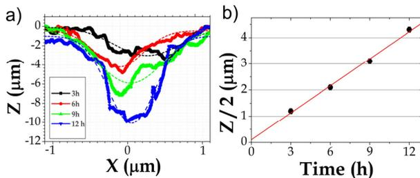
Figure 3: Depth profiles,  $Z$ , of the Cu surface along the  $X$  axis after 5 keV  $\text{Ar}^+$  irradiation for 3-12 h with Gaussian fit curves (a) and the half maximum of the crater depth vs. time (b).
