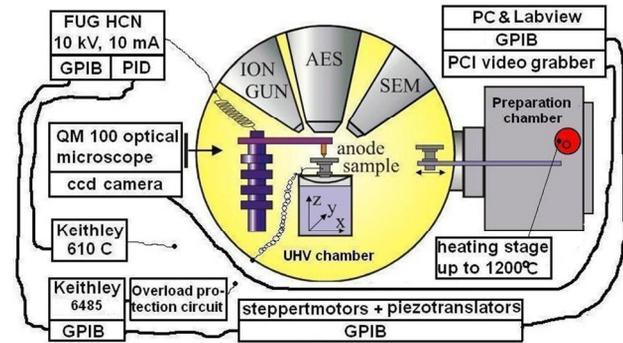
Figure 1: Schematic view of the field emission scanning microscope.
