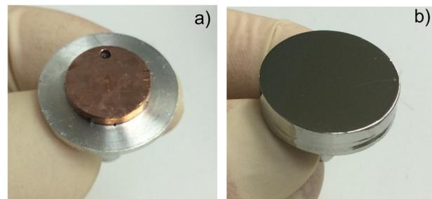
Figure 2: Images of polycrystalline Cu sample fixed on an Al holder (a), and a large-grain Nb sample (b).
