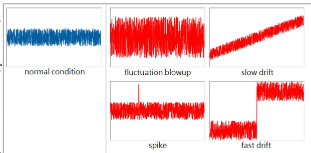
Figure 2: Display of signals in the TPS SR when abnormal conditions.
