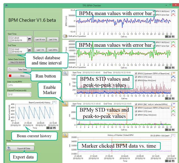
Figure 1: The graphical interface of BPM checking software.
