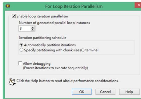
Figure 3: The key setup page for setting parallelism execution in LabVIEW.
