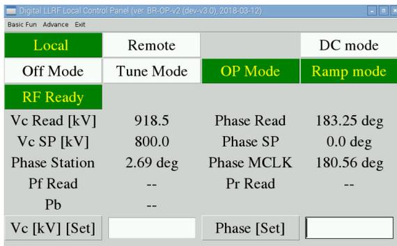
Figure 3: The booster RF GUI for the local operation.
