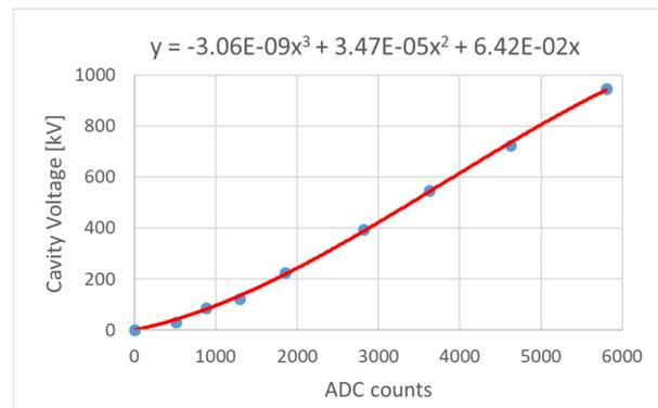
Figure 4: A 3<sup>rd</sup> order polynomial fit for the cavity voltage calibration.
