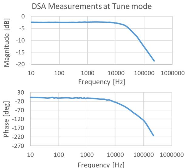
Figure 8: DSA measurements of the TPS booster RF in tune mode with a cavity voltage of 650 kV.
