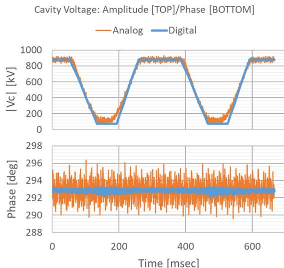
Figure 6: Cavity voltage amplitude and phase during routine operations of the TPS booster RF measured by the analog and digital LLRF systems.
