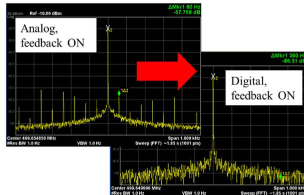
Figure 5: The cavity field spectrum at the operation mode with cavity voltage of 950 kV before (left) and after the DLLRF system (right) installed.
