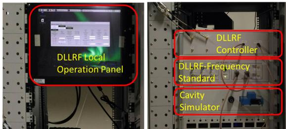
Figure 2: Photos of the DLLRF system. Upper (left) and bottom (right) layers of the rack.
