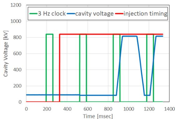
Figure 7: Related signals as obtained from the transient data recorder in the energy savings mode using a test signal.
