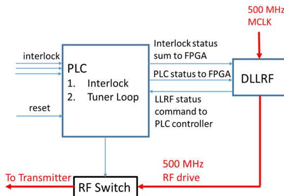
Figure 1: Hardware architecture of the DLLRF system.
