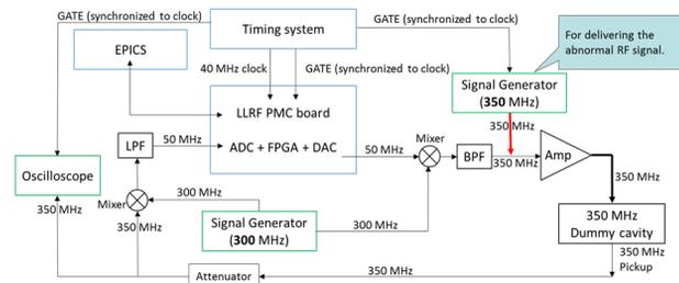
Figure 4: Test bench for testing the RF interlock logic.
