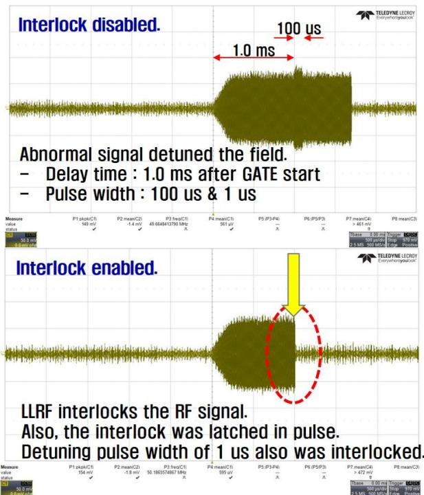
Figure 5: Test result of digital RF interlock logic. (upper) RF interlock disabled. (lower) RF interlock enabled.
