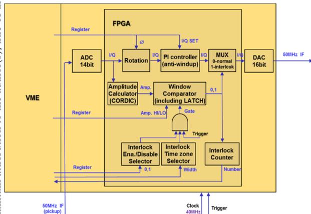
Figure 3: Digital RF interlock logics in the FPGA.
