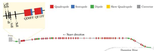
Figure 1: Schematic of the layout of the ATF2 extraction line and final focus [1], with the FONT IP region enlarged.
