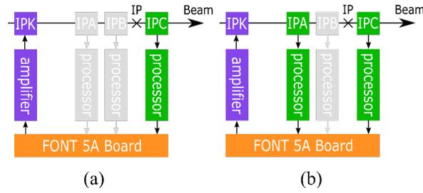
Figure 3: Diagrams of feedback loops with cavity BPMs (IPA, IPB and IPC) and a stripline kicker (IPK) for (a) single-BPM feedback with beam stabilisation at IPC and (b) two-BPM feedback, with position measurements at IPA and IPC, for beam stabilisation at an intermediate location.
