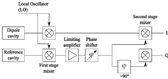
Figure 2: Simplified schematic of the FONT processing electronics [3].
