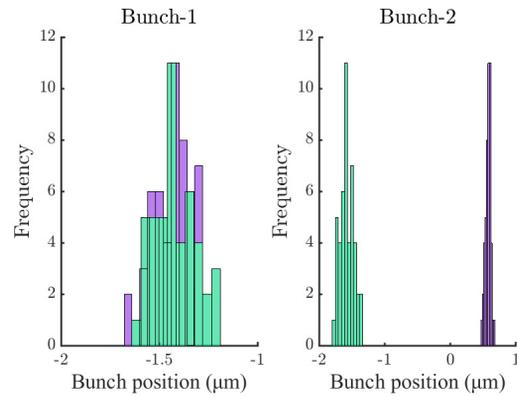
Figure 5: Distribution of bunch positions measured at IPB, with two-BPM feedback off (green) and feedback on (purple). The position jitters are given in Table 2.
