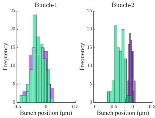
Figure 4: Distribution of bunch positions measured at IPC, with single-BPM feedback off (green) and feedback on (purple). The position jitters are given in Table 1.
