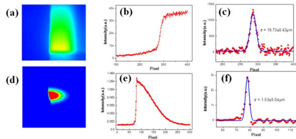
Figure 2: Image of tungsten bar edge observed in X-ray fan with (a) cam1 and (d) cam2. Profile of the edge of (b) cam1 and (e) cam2. The derivative of the profile (red) and a fitted Gaussian curve (blue) of (c) cam1 and (f) cam2.
