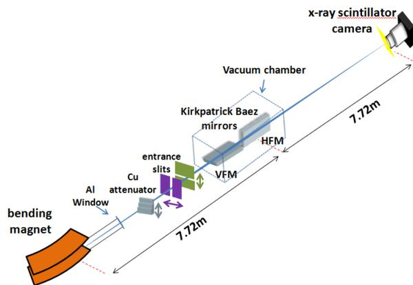
Figure 1: Schematic diagram of KB mirror system.
