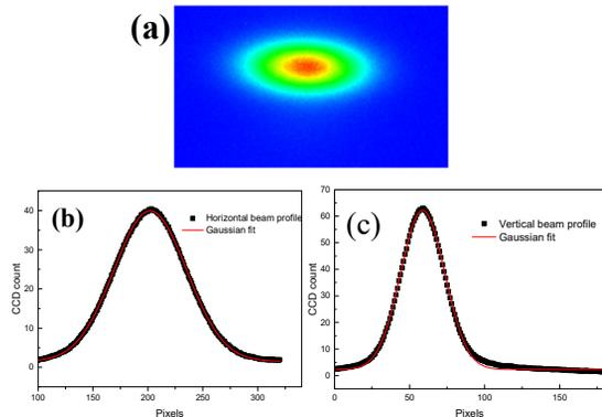
Figure 3: (a) Observed image of the KB mirror monitor in the SSRF control room.(b) Horizontal and (c) vertical beam profiles with their fitted gaussian curves.
