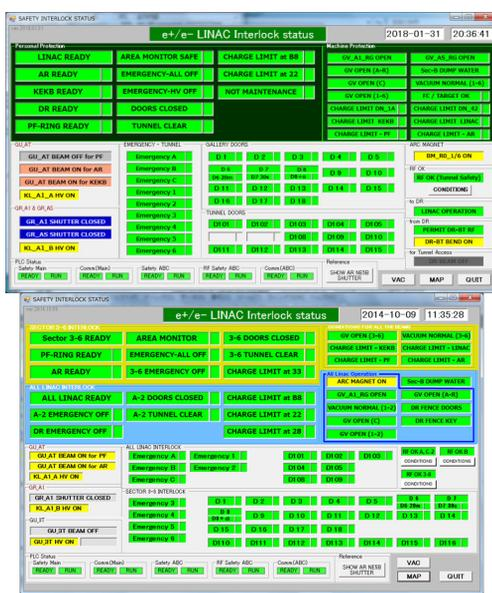
Figure 4: Image example of Interlock status display after system update (top) and before system update (bottom).
