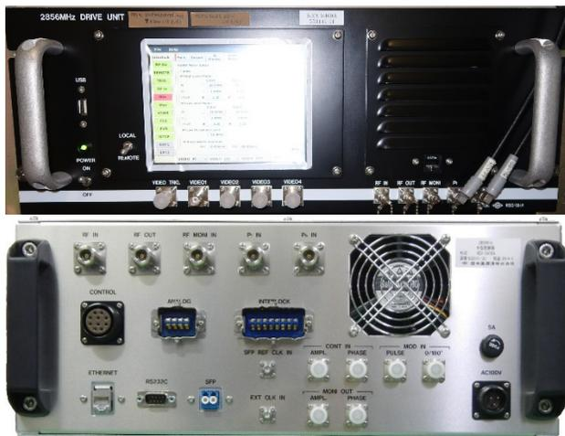
Figure 4: Front/rear panel of LLRF control unit.
