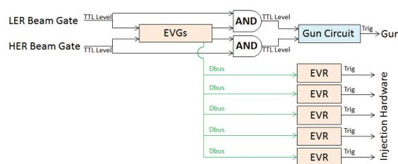
Figure 2: Schematic view of Beam Gate circuit: the output for electron gun is provided as the level signal while others are provided as the Dbus.
