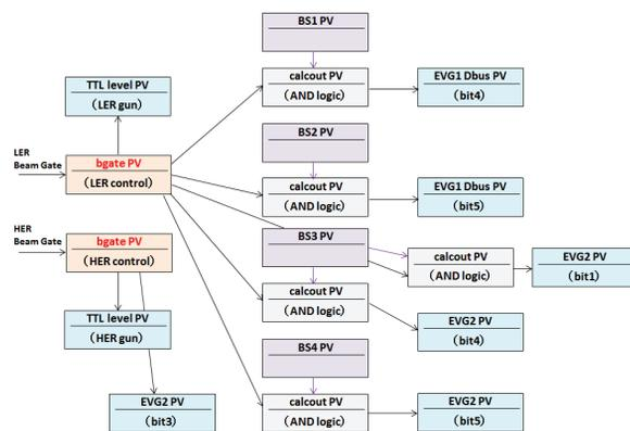
Figure 3: Flow chart of Beam Gate core process on EPICS IOC: it consists of bgate PVs, reflective memory PVs, and calcout PVs configured as “AND” logic.
