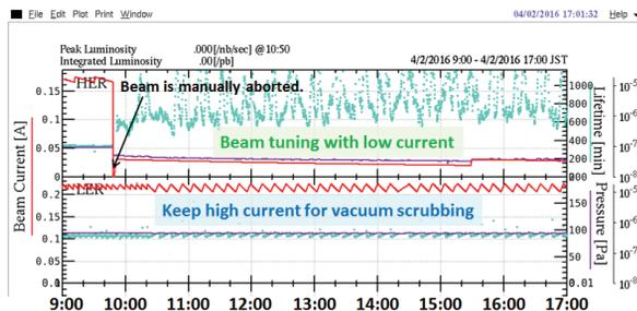
Figure 1: Example of beam operation: the beam currents at LER and HER are plotted. The high beam current at LER is kept by iterating the open and close of Beam Gate.
