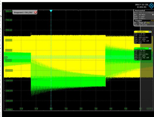
Figure 6: Step-wise detuning caused by microphonics driving five mechanical eigenmodes (green) and its effect on the transmitted voltage (yellow).
