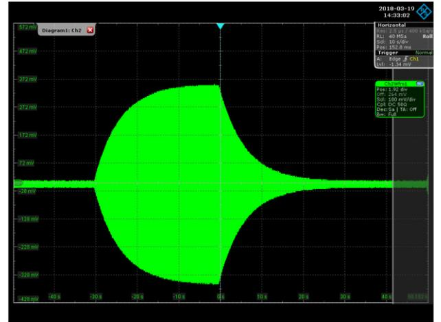
Figure 3: Transmitted voltage for  $Q_{ext} = Q_0 = 5 \times 10^{10}$ ,  $\frac{r}{Q} = 1000$  ohm,  $\Delta f = 0$ ,  $f_{RF} = 1.3$  GHz, and a pulse length of 30 s. The frequency of the signal is 25 MHz.
