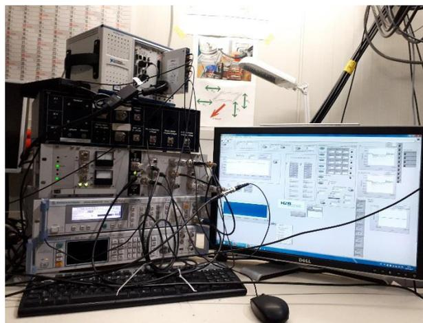
Figure 7: PXI running the cavity simulator (top), up/down-converter (center), signal generators (bottom) and GUI (right).
