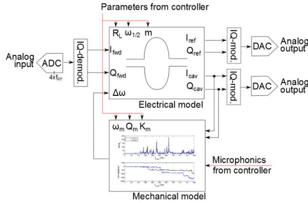
Figure 2: Block diagram of the implementation.
