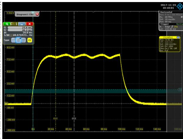
Figure 5: Effect of the Lorentz force detuning coupled with a 50Hz mechanical mode in the amplitude in a cavity with  $Q_0 = 5 \times 10^{10}$ ,  $Q_{\text{ext}} = 5 \times 10^7$ , and  $f_{RF} = 1.3$  GHz.
