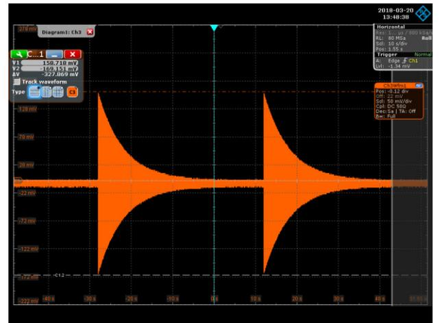
Figure 4: Reflected voltage for  $Q_{ext} = Q_0 = 5 \times 10^{10}$ ,  $\frac{r}{Q} = 1000$  ohm,  $\Delta f = 0$ ,  $f_{RF} = 1.3$  GHz, and a pulse length of 40 s. The frequency of the signal is 25 MHz. The peaks at the beginning and end of the pulse have the same height as it is a critical coupled cavity.
