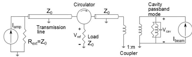
Figure 1: Electrical equivalent circuit of a superconducting cavity.
