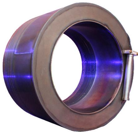
Figure 2: Completed niobium CCC-XD with anodized surface, an inner diameter of 250 mm, an outer diameter of 350 mm, a thickness of the niobium walls of 3 mm, a height of 207 mm, and a weight of 56 kg.
