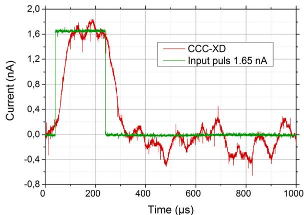
Figure 5: Single pulse signal response of the CCC-XD (SQUID electronics with 10 kHz low-pass filter) compared to the 1.65 nA input signal (Device: Data Sys 7000 Digital Storage Oscilloscope) [4].
