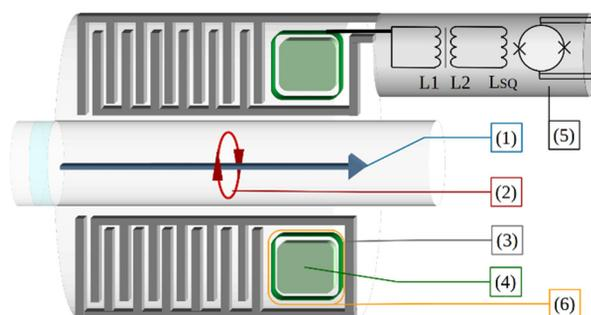
Figure 1: Components of a CCC as used in accelerators (1) Charged particle beam with (2) azimuthal magnetic field, (3) meander shielding as magnetic field filter, (4) pick-up coil and flux concentrator, (5) SQUID cartridge (6) calibration wire.
