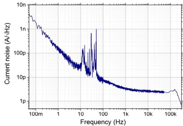
Figure 3: Noise measurements (Devices: HP 35670A Signal Analyzer 50 kHz, HP 89410A Vector Analyzer 10 MHz).
