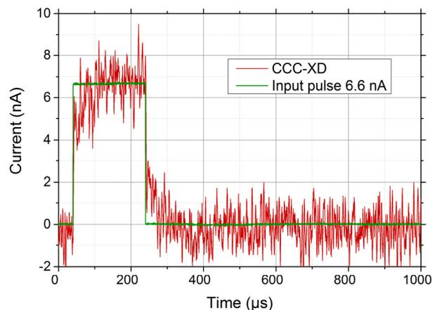
Figure 4: Single pulse signal response of the CCC-XD (SQUID electronics without 10 kHz low-pass filter) compared to the 6.6 nA input signal (Device: Data Sys 7000 Digital Storage Oscilloscope) [4].
