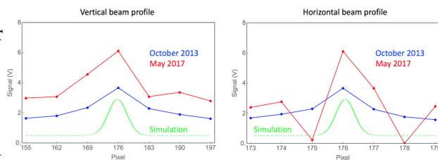
Figure 2: Observed beam signal on the monitor. The signal is taken from only one array of column (vertical) and row (horizontal) across the beam center pixel in the monitor. Some pixel has a low signal gain or lost a gain at all.
