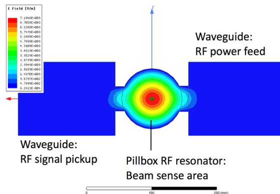
Figure 7: Conceptual design of a new prototype RF detector.
