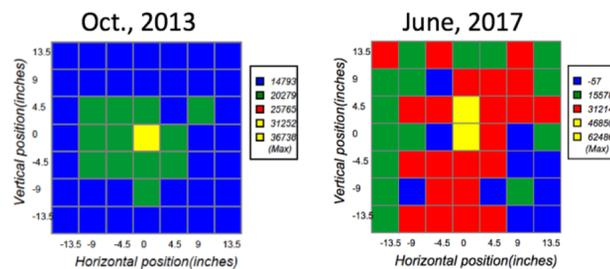
Figure 1: The position beam profile on the NuMI hadron monitor.
