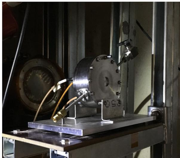
Figure 4: The fabricated RF test cavity on the SY beam line. The SEM behind the cavity is used to measure the beam intensity.
