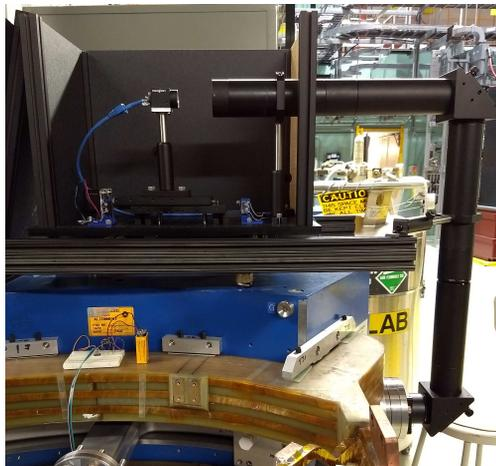
(a) Prototype mounted on 60 degree magnet
