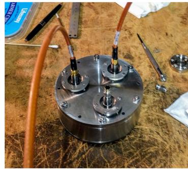
Figure 5: Tunable Q-factor Radio-Frequency cavity.
