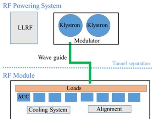
Figure 3. Simplified layout of the Klystron based powering design.
