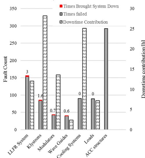
Figure 4. Components failure number and downtime contribution in one year of operation for the Drive Beam based powering.
