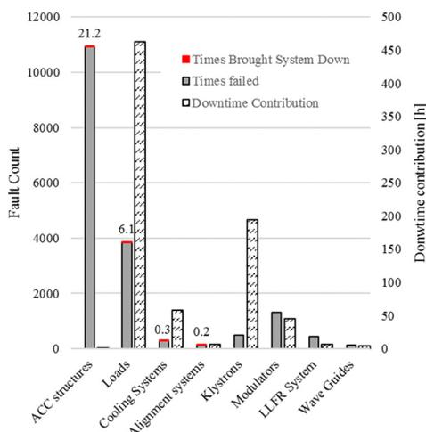
Figure 5. Components failure number and downtime contribution in one year of operation for the Klystron based powering.
