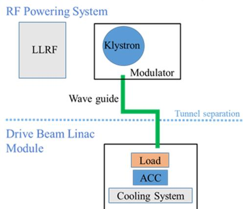
Figure 2. Simplified layout of the Drive Beam based powering design.
