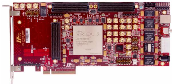
Figure 3: HTG-700 Virtex-7 FPGA Board.
