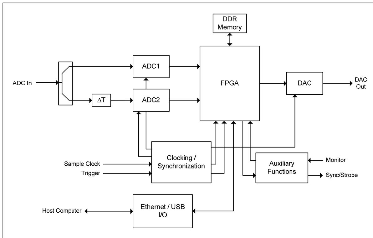
Figure 4: The Architecture of the 8GSa/s Ultrawideband Feedback Processor.
