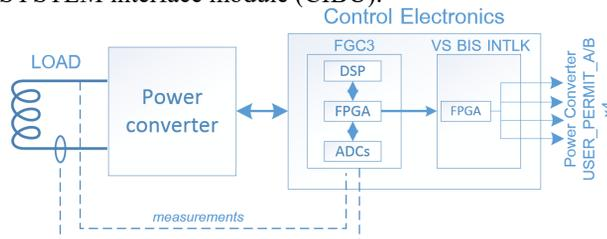
Figure 3: Hardware implementation of power converter user permit.
