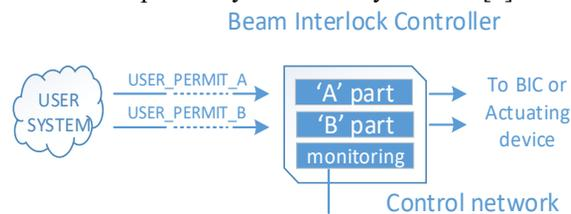
Figure 1: Simplified diagram of user system to BIS interface.
