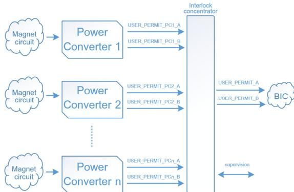
Figure 4: Power Converter permit concentrator.
