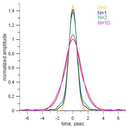
Figure 6: Original bunch distribution (red), first iteration (yellow) and 10<sup>th</sup> iteration (pink).
