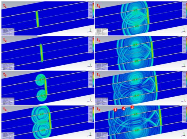
Figure 4: CST simulation of a 1 ps beam passing by two 200-micron beam-pipe breaks separated by 0.5 mm. Consequent shots at times  $t_1, t_2, \dots, t_8$  are presented. There is interference between the excited pulses that can be measured with a detector array. The detector array location is shown on the  $t_8$  plot with red circles.
