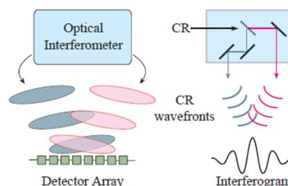
Figure 2: From [7]. Conceptual scheme of the real-time interferometer (RTI) which autocorrelates the phase fronts of a beam-based coherent radiation source to determine bunch length information.
