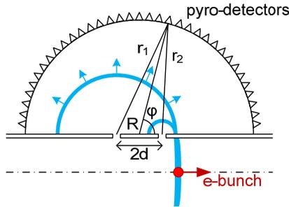
Figure 3: Non-invasive bunch length measurement setup.
