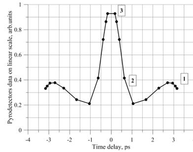
Figure 5: Pyro-detector's output for various time delay pairs, i.e. autocorrelation function.
