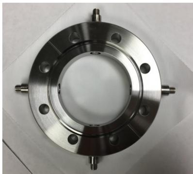
Figure 1: The in-flange simplified button-type BPM pickup device.
