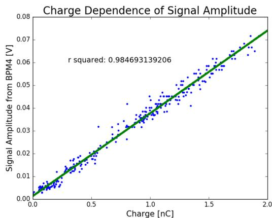
Figure 2: The combined signal strength of four electrodes of the in-flange pickup device, as a function of charge.
