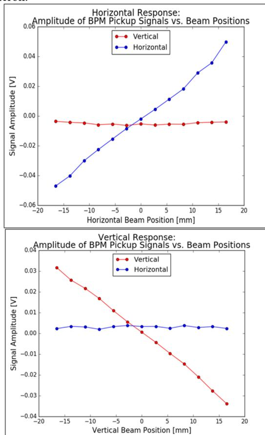
Figure 3: The difference in signal amplitudes of the opposite electrodes as a function of the horizontal (vertical) beam position.
