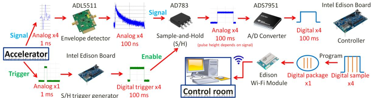
Figure 4: The mockup wireless BPM system using the COTS Intel Edison board.
