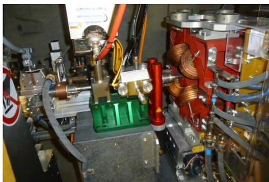
Figure 4: BLMs in undulator section.
