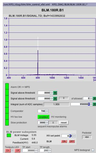
Figure 5: BLM panel in the control system, one bunch; the small hump between 800us and 1200us is darkcurrent.
