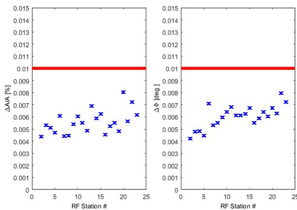
Figure 2: In-loop intra-pulse amplitude (left) and phase (right) stability of the XTL RF stations averaged over 1000 pulses as of 23rd of June 2017. The red line indicates the required stability level.
