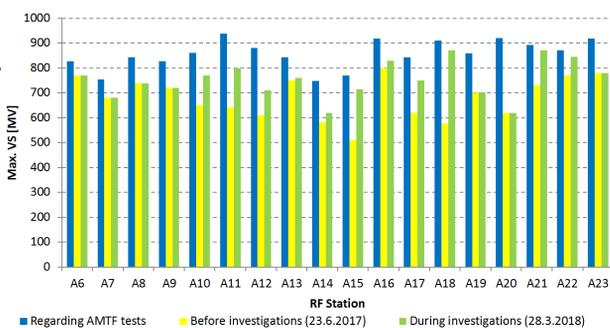
Figure 3: Maximal VS gradients of L3: estimated from AMTF tests (blue), measured at XFEL on the 23rd of June 2017 (yellow) and on the 28th of March 2018 (green) during the maximum energy reach investigations.
