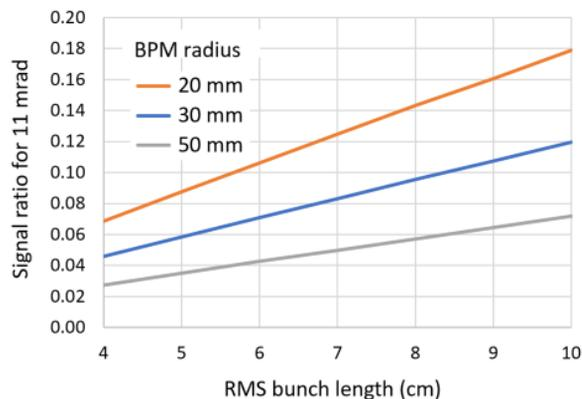
Figure 7: Signal ratio as function of RMS bunch length for three BPM radii.
