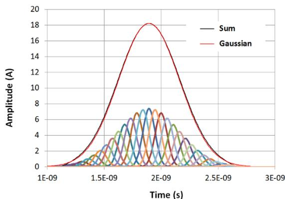
Figure 3: 27 bunches used as input to simulate the 8 cm RMS crabbed bunch. The individual bunches have a 1.6 cm RMS width, they are displaced laterally according to the pattern shown in Fig. 1B and their sum approximates a 8 cm RMS, 12.5 nC Gaussian crabbed bunch.
