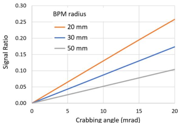
Figure 6: Signal ratios  $(A_0 - B_0)/(A_{max} + B_{max})$  as function of crabbing angles for three BPM radii.
