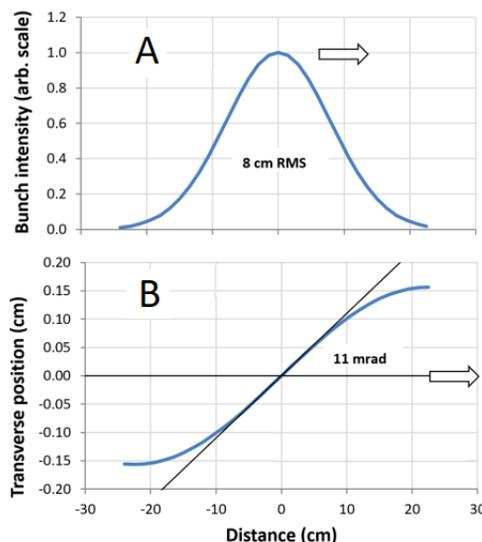
Figure 1: Bunch intensity (A) and transverse position (B) of an 8 cm RMS bunch crabbled at an angle of 11 mrad by a 336 MHz cavity.
