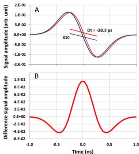
Figure 2: A) Signals induced on two opposite BPM PUEs by the bunch described in Fig. 1. B) Difference of the signals shown in A) normalized to the average of the peak values.
