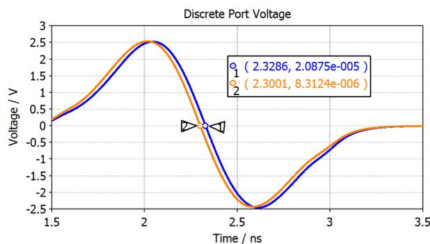
Figure 4: Particle Studio output for the two, opposite, horizontal PUEs when using a 60 mm diameter BPM with 10 mm diameter PUEs with a simulated crabbed bunch input described in Fig. 3.
