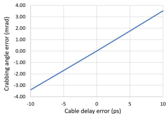
Figure 9: Crabbing angle errors as function of cable delay variations.
