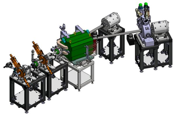
Figure 1. Layout of the RFQ/SCDTL test bench. Beam enters from the left. The DBoxes, BPMs, Phase Probes, EM quadrupoles, spectrometer dipole and end Faraday cups are shown.
