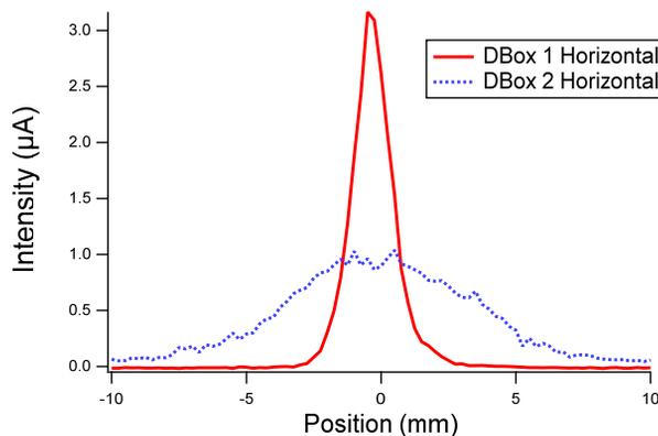
Figure 3. Horizontal beam profiles taken at the two DBoxes of the test bench placed after the SCDTL1.
