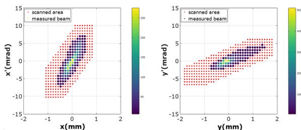
Figure 4. Transverse phase space of the 5 MeV beam, measured by the two DBoxes of the test bench. Horizontal plane on left, vertical plane on right. Red points show the measured phase space area; colour map shows the points with measured beam above 5 nA.
