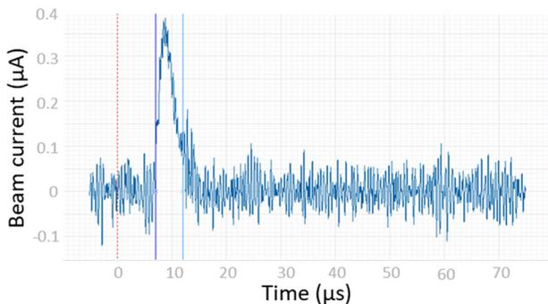
Figure 2. Faraday cup measurement of weak ( $\sim 400$  nA) beam, taken with the highest gain setting and illustrating the extremely low noise and high time resolution. The red vertical line represents the trigger for the BD acquisition crate, the two blue vertical lines are a selectable integration window used by the profile and emittance procedures.
