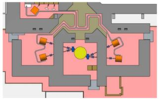
Figure 2: Layout of ACE Isotopes, showing the cyclotron vault (middle), production vaults (left and right) and the proposed target transport system.
