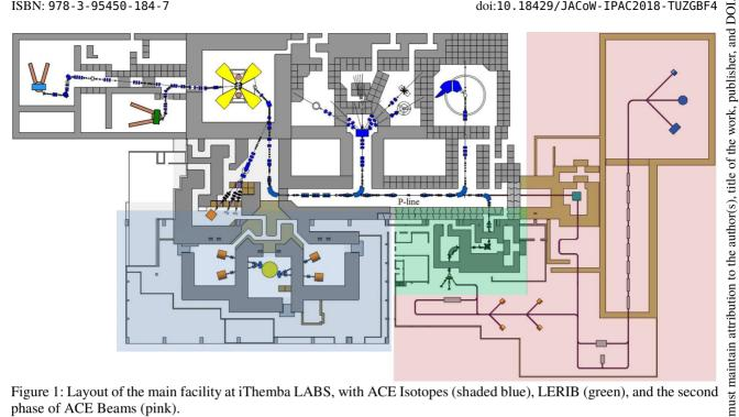
Figure 1: Layout of the main facility at iThemba LABS, with ACE Isotopes (shaded blue), LERIB (green), and the second phase of ACE Beams (pink).
