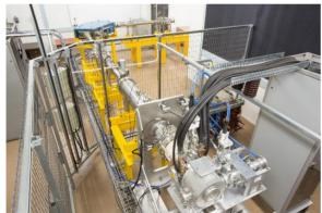
Figure 4: The LERIB test-bench contains a target/ionsource (foreground) on a high-voltage platform, and a beam line with an analysing magnet (background).
