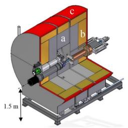
Figure 3: Cutaway view of the production station, with the beamline (left) and cooling-water pusher arm (right). The shielding consists of (a) an inner iron layer, (b) borated paraffin wax and (c) an outer lead shield.
