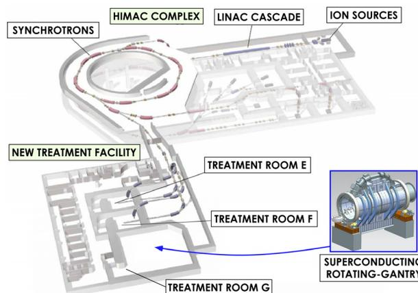
Figure 1: Bird's eye view of the HIMAC complex. The HIMAC complex consists of three ion sources, one linac cascade, two synchrotron rings, and three treatment rooms. The new treatment facility was constructed in conjunction with the HIMAC complex, and has the three treatment rooms.
