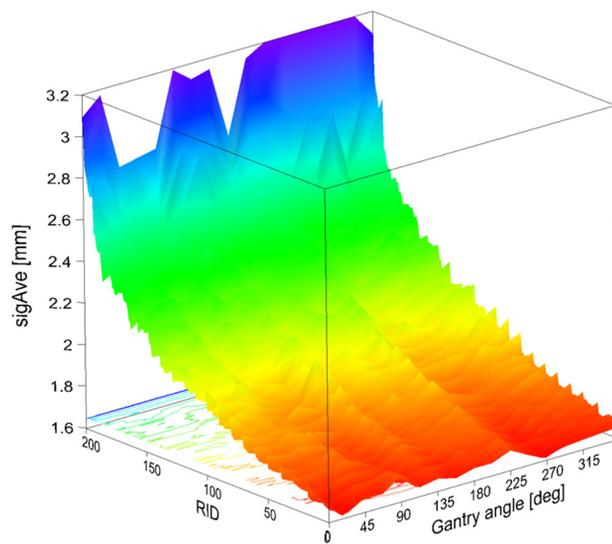
Figure 6: Measured  $1\sigma$  beam size as a function of the gantry angle and RID. The RID corresponds to the beam energy ID; RID=0 for  $E=430$  MeV/ $u$  and RID=200 for  $E=56$  MeV/ $u$ . The beam size was obtained by averaging those for the horizontal and vertical coordinates.
