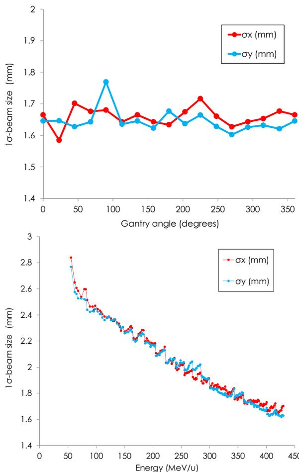
Figure 5: Measured  $1\sigma$  beam sizes for the horizontal and vertical coordinates at the isocenter as functions of the gantry angle (upper) and beam energy (lower).
