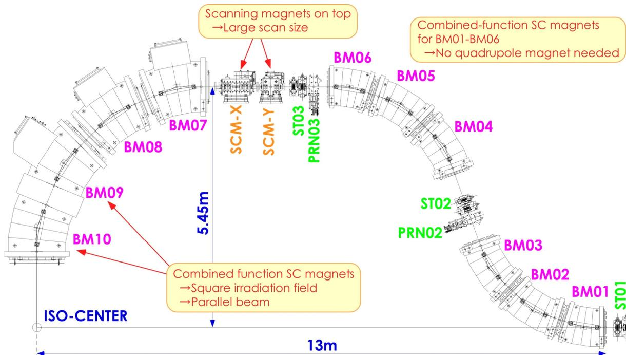
Figure 2: Layout of the superconducting rotating-gantry. The gantry consists of the ten superconducting magnets (BM01-BM10), the three pairs of the steering magnets (ST01-ST03) and profile monitors (PRN01-PRN03), and a pair of the scanning magnets (SCM-X and SCM-Y).
