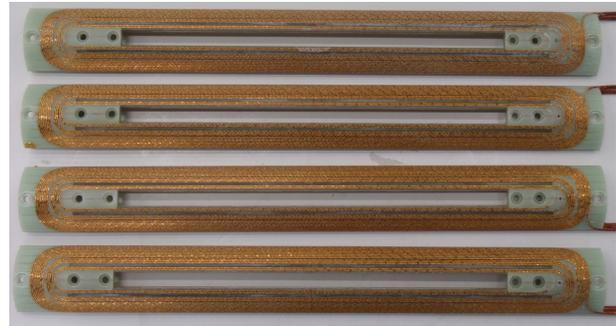
Figure 6: Four SC coils for QC1LP.
