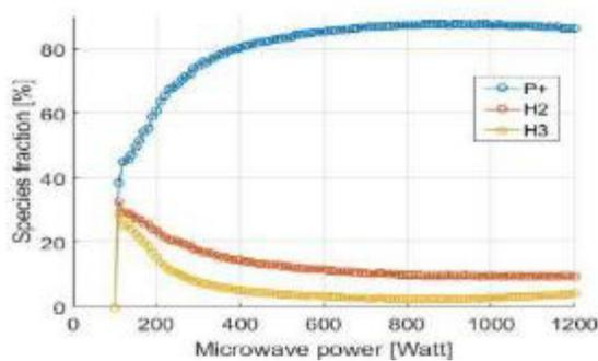
Figure 3: Proton fraction produced vs. microwave power at nominal source configuration.
