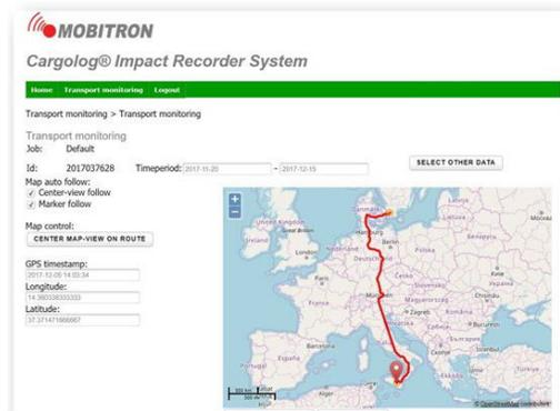
Figure 8: GPS web monitoring user interface.
