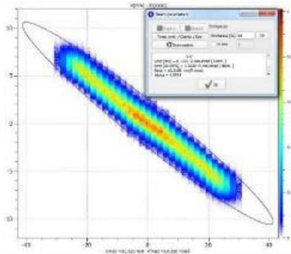
Figure 7: Emittance measurement at the center of the LEBT.
