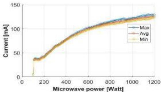
Figure 2: Total current vs. microwave power at nominal source configuration.
