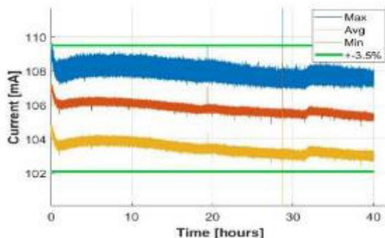
Figure 4: Pulse to Pulse stability at nominal source configuration.
