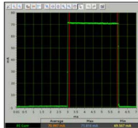
Figure 5: Beam pulse measurement with a Faraday Cup located after the LEBT-RFQ beam lattice interface, the first three milliseconds of beam produced by the source are stopped by using a chopper in the LEBT.
