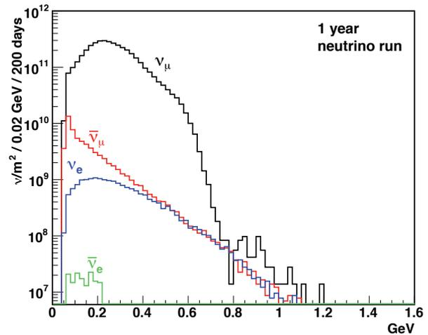
Figure 3: Neutrino energy distribution at a distance of 100 km on-axis from the target station, for 2.0 GeV protons and positive horn current polarity.
