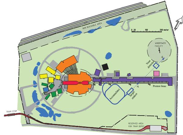
Figure 2: Layout of the ESS installation with a possible neutrino facility implementation (accumulator, target station, near detector).
