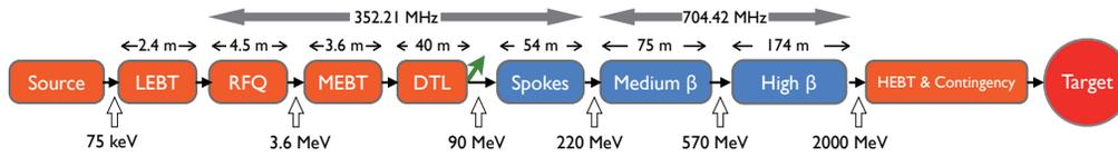
Figure 1: Schematic view of the ESS proton linac.
