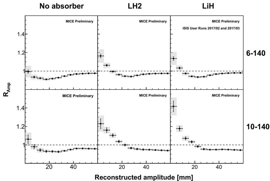
Figure 3: The ratio,  $R_{\text{Amp}}$ , of the downstream and upstream samples for (left) an empty channel, (middle) liquid hydrogen, and (right) lithium hydride. The ratios are shown for two input beam line settings, with a nominal momentum of  $p = 140 \text{ MeV}/c$  and nominal emittance of 6 (top), and 10 mm (bottom). Cooling is seen where  $R_{\text{Amp}} > 1$ . Statistical uncertainties are given as bars, systematic uncertainties (grey) are under study.
