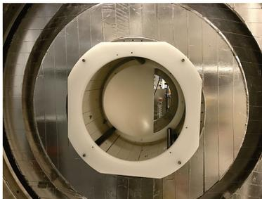
Figure 4: Wedge absorber as assembled inside the focus coil module right before data taking.
