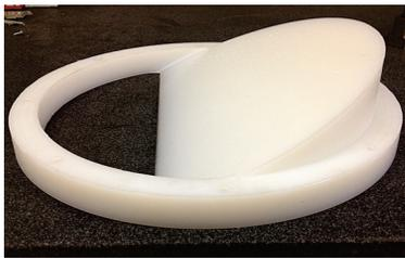
Figure 3: Half-wedge as manufactured at the University of Mississippi. The full wedge consists of two half-wedges. The resulting wedge has a 45-degree opening angle and on-axis length of 52 mm.
