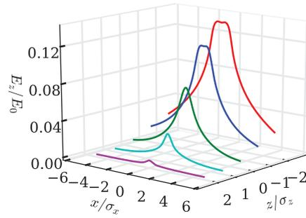
Figure 4: Distribution of  $E_z^b$  on the  $x-z$  plane:  $z > 0$  for the bunch head.
