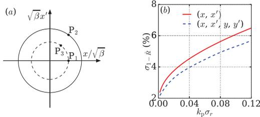
Figure 2: (a) Illustration of particle's motion in 2D normalized trace space and (b) dependence of slice energy spread on the normalized beam size in 2D and 4D trace space.
