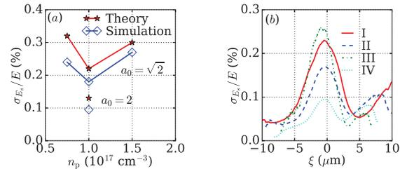
Figure 3: (a) Slice energy spread at the bunch center ( $\xi = 0$ ) as a function of the plasma density and laser strength; (b) slice energy spread distributions for  $a_0 = \sqrt{2}$  and  $n_p = 0.5, 1.0, 1.5 \times 10^{17} \text{ cm}^{-3}$  (I to III) and for  $a_0 = 2$  and  $n_p = 1.0 \times 10^{17} \text{ cm}^{-3}$  (IV).
