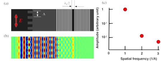
Figure 3: A structure of multi-layered F-P DLA (a), the map of the longitudinal electric field strength  $E_z$  (b) and the Fourier spectrum of  $E_z$  (c).
