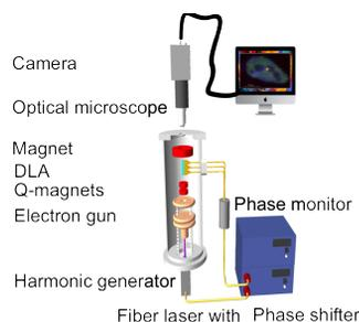
Figure 1: The concept drawing of the compact EMBI system for the radiobiology research.
