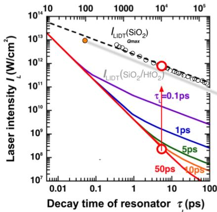
Figure 2: The energy enhancement in optical cavities is shown by the red arrow for  $Q = 10000$ . The broken line and the gray line are LIDTs of the bulk  $\text{SiO}_2$  and the multi-layer mirror of  $\text{SiO}_2$  and  $\text{HfO}_2$ , respectively.
