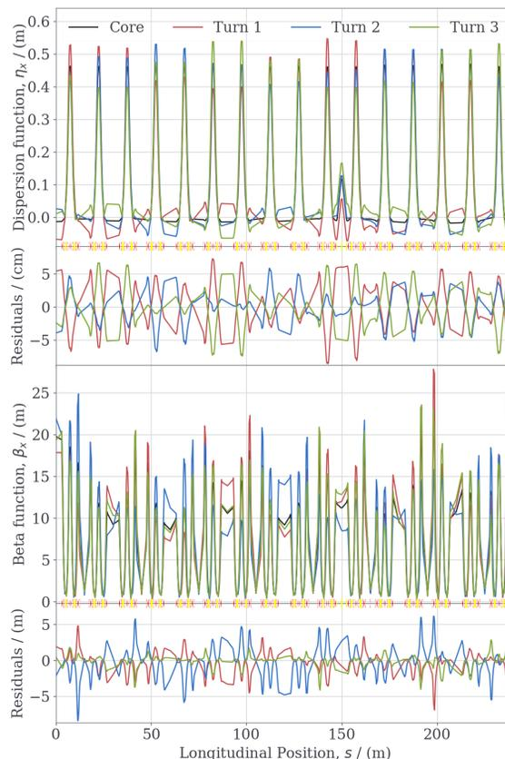
Figure 1: Dispersion and betatron function of the BESSY II TRIBs optics and the residuals to the core orbit. [11, 12]
