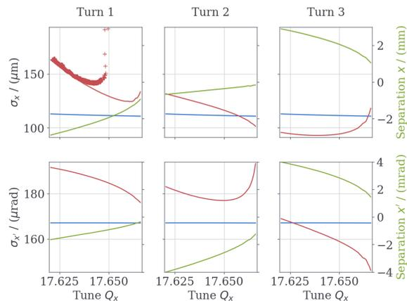
Figure 6: These plots show the core (blue line) and island (red line) beam size as well as the separation (green line) of the two for each turn (or spot) of the island orbit at the position of a pinhole monitor as a function of the core tune. The measured Beam size (red crosses, upper left subplot) of the first island shows similar behavior as the simulated. The Position of the minimum differs and needs to be investigated further. [11, 12]
