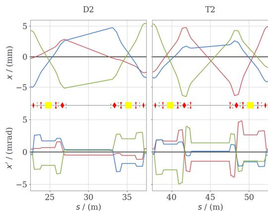
Figure 2: Exemplary spatial and angular separation of the island orbit in a triplet and doublet section. [11, 12]
