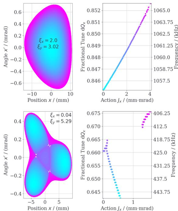
Figure 4: The TSWA for the BESSY II Standard User (upper plot) and the BESSY II TRIBs (lower plot) optics from transverse tracking simulations. The impact of chromaticity and energy spread is not included. [11–13]
