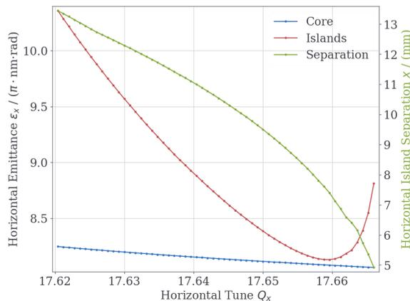
Figure 5: Emittance of the island (red) and core (blue) orbits as a function of the core tune. The maximum separation of the island and core orbits over the entire ring (green) is determined from the core tune and the TSWA. [11, 12]
