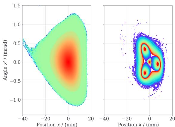
Figure 3: Horizontal phase space of the LOCO measured BESSY II standard user and TRIBs optics showing the proportions of their dynamic apertures. The particles are colored according to their initial position. [11–13]
