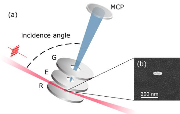
Figure 1: (a) VMI spectrometer consisting of three electrodes: repeller (R), extractor (E) and ground (G); (b) SEM image of the 75- $\mu\text{m}$  pitch field-emitter array of Au nanorods.
