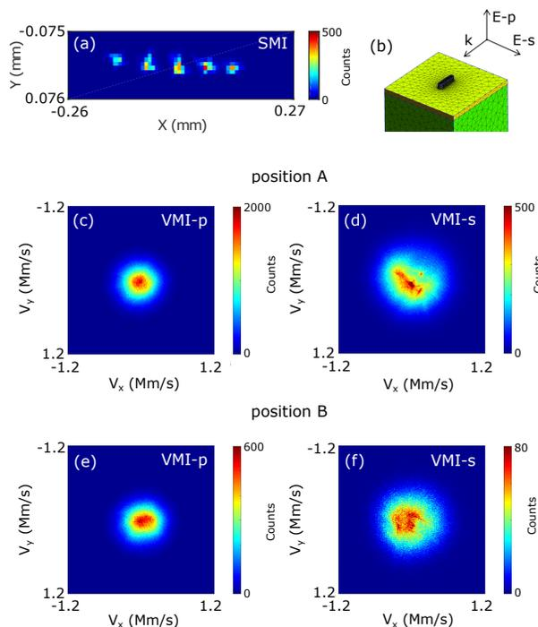
Figure 2: (a) SMI image of a 75- $\mu\text{m}$  pitch field-emitter array of Au nanorods; (b) sketch of laser polarization with respect to the experiment, where E-p and E-s denote the electric field directions under p- and s-polarization, respectively; VMI images of position A under (c) p-polarization and (d) s-polarization; VMI images of position B under (e) p-polarization and (f) s-polarization.
