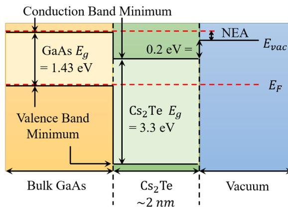
Figure 1: Energy band diagram of GaAs activated with Cs<sub>2</sub>Te. The vacuum level is below the conduction band minimum of bulk GaAs, indicating achievement of NEA. GaAs band gap energy photons (1.43 eV) excites electrons only from the bulk valence band minimum because of large band gap (3.3 eV) of Cs<sub>2</sub>Te.
