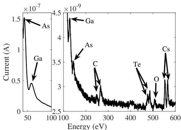
Figure 3: Auger electron spectrum of GaAs activated by  $\text{Cs}_2\text{Te}$ .
