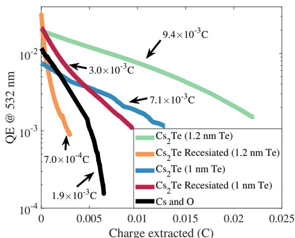
Figure 5: Quantum Efficiency measured at 532 nm as a function of extracted charges for various activation methods of GaAs. The charge lifetimes calculated from exponential fits are written next to each curve.
