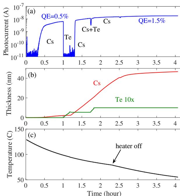
Figure 2: (a) Photocurrent measured over time using a 532 nm laser shining GaAs during the growth of  $\text{Cs}_2\text{Te}$ ; (b) Estimated thicknesses of Cs and Te deposition from the quartz microbalance frequency shift; (c) Temperature of GaAs substrate during the  $\text{Cs}_2\text{Te}$  growth.
