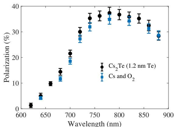
Figure 6: Comparison of photoelectron spin-polarization from GaAs prepared with  $\text{Cs}_2\text{Te}$  activation and standard activation with Cs and  $\text{O}_2$ .
