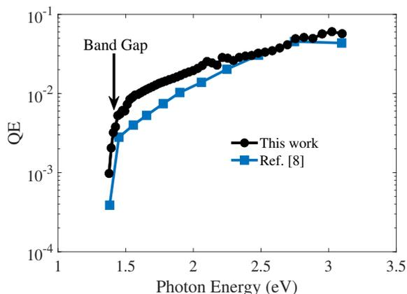
Figure 4: Spectral response of GaAs activated with  $\text{Cs}_2\text{Te}$  in this work compared to the one from Ref. [8].
