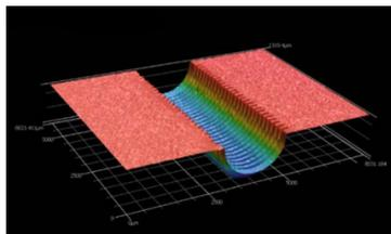
(b) Profile of corrugated waveguide measurement
