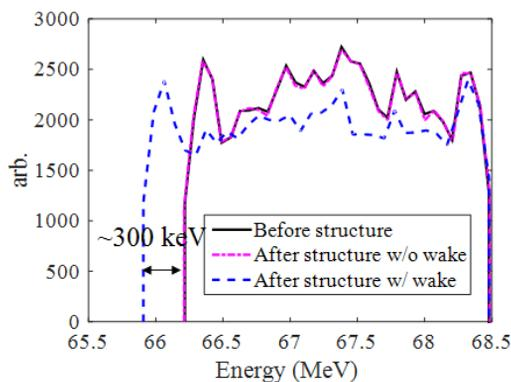
Figure 6: Energy of the beam at simulated spectrometer with and without corrugated waveguide.
