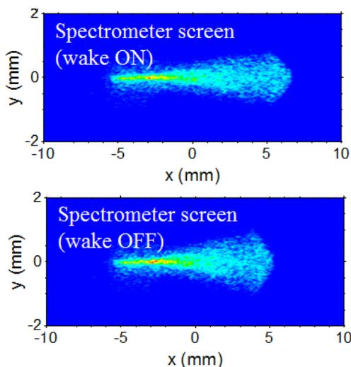
Figure 7: Simulation results of beam spread at spectrometer with and without corrugated waveguide.
