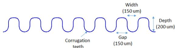
Figure 1: Corrugated waveguide cross-sectional input geometry for ECHO.
