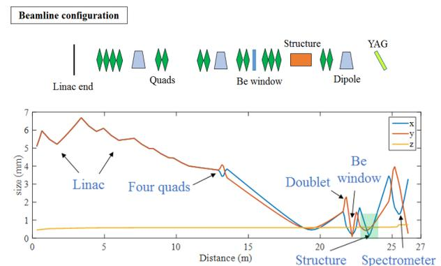
Figure 5: Argonne Wakefield Accelerator lattice layout.
