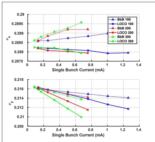
Figure 3: Tune shift for different fill patterns plotted against the equivalent single bunch current in the storage ring. The changing gradient for both measured and LOCO tune gradients shows the effect is unrelated to the single bunch current.
