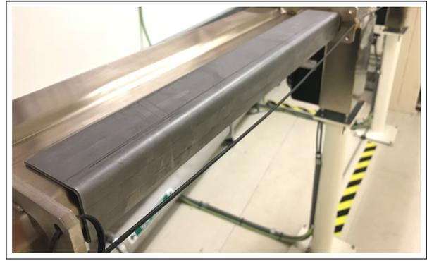
Figure 2: 3 mm thick ferro-magnetic capping made from mild steel (250 grade).
