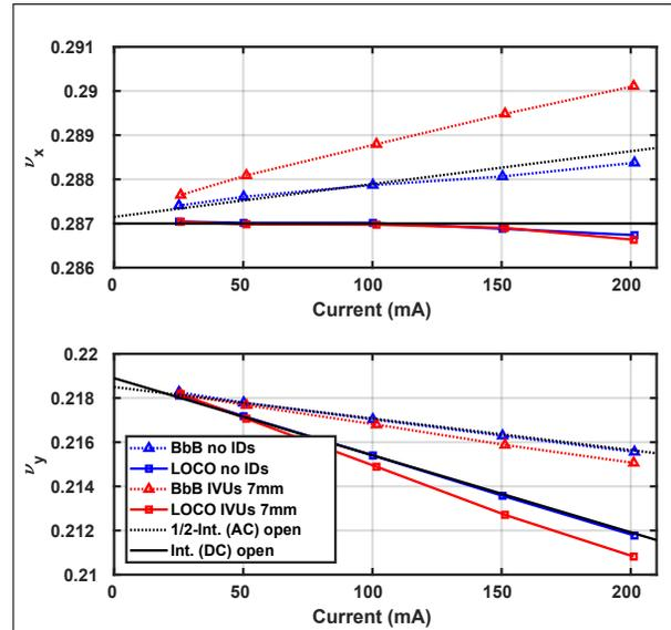
Figure 1: Tunes measured with the BbB system and LOCO derived tunes. The measured and LOCO derived tune gradients are completely different and both clearly display an effect resulting from closing the IVU gap.
