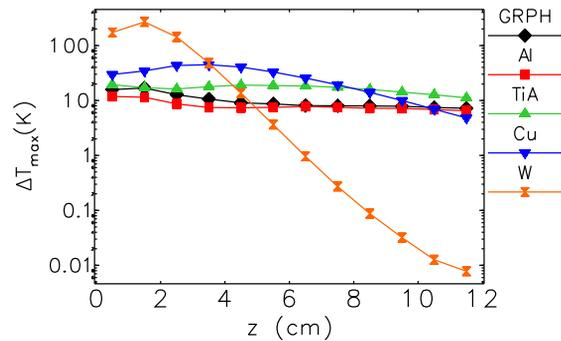
Figure 4: Longitudinal peak  $\Delta T$  distributions for a single decohered bunch, based on MARS simulations.
