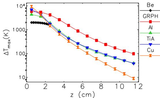
Figure 3: Longitudinal peak  $\Delta T$  distributions for a single bunch without decoherence, based on MARS simulations.
