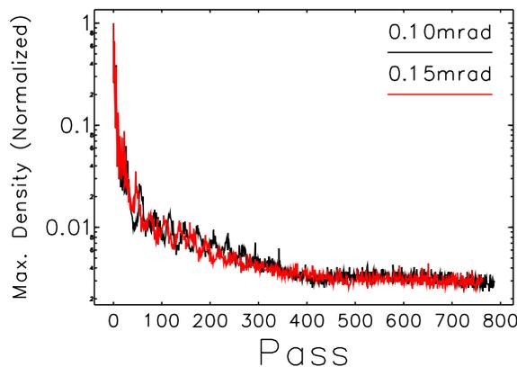
Figure 1: Maximum particle density in bunch 0 as a function of the number of turns since the vertical kick.
