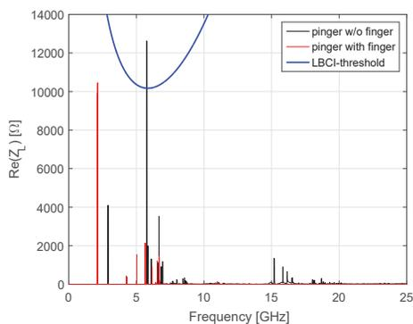
Figure 5: Pinger impedance with and without fingers.
