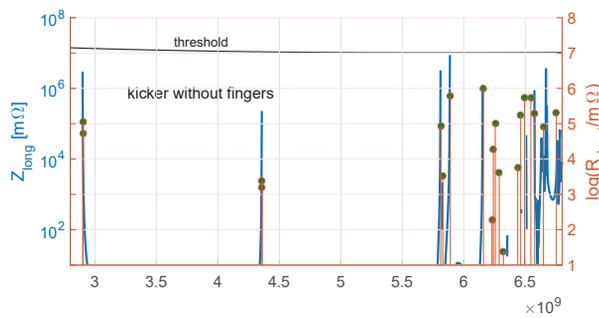
Figure 7:  $Re(Z_L)$ (blue) &  $R_s$  of the eigenmodes (orange).
