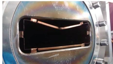
Figure 3: Collapsed RF-finger .
