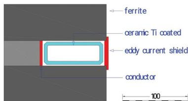
Figure 1: Cross section of Storage Ring injection kicker.
