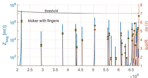
Figure 6:  $Re(Z_L)$ (blue) &  $R_s$  of the eigenmodes (orange).
