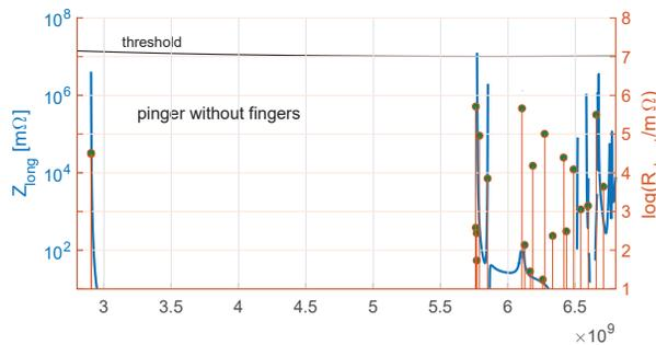
Figure 9:  $Re(Z_L)$ (blue) &  $R_s$  of the eigenmodes (orange).
