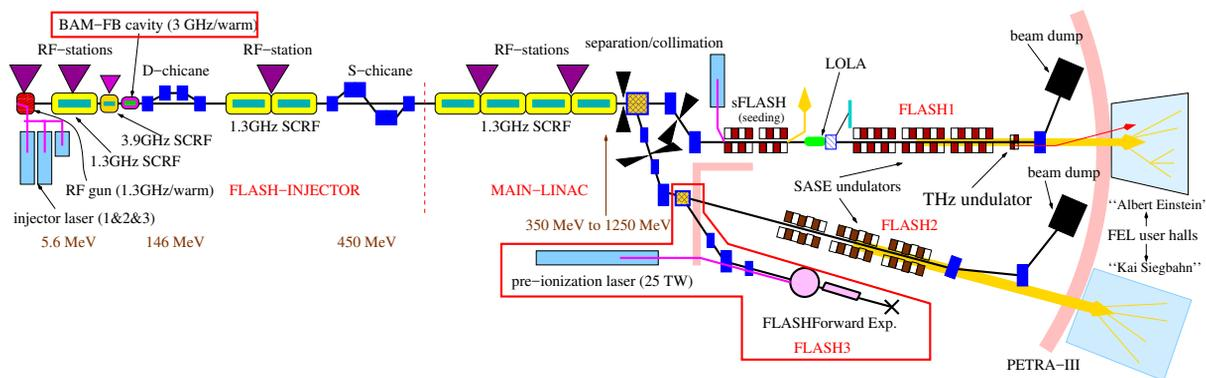
Figure 1: The FLASH facility (not to scale).
