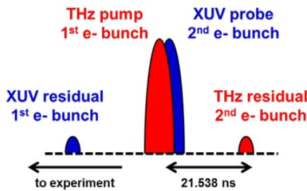
Figure 2: XUV/THz Pulse structure with active THz (injector laser) Pulse doubler.
