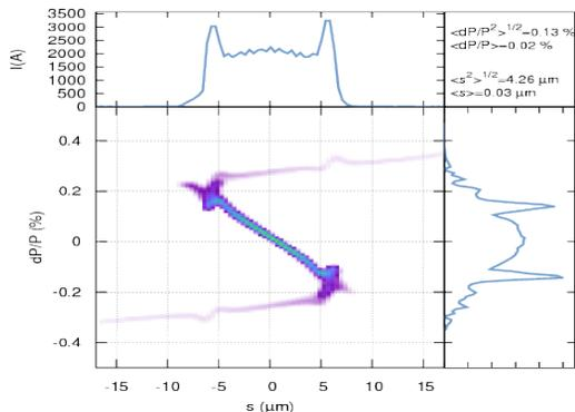
Figure 5: Long. PS: 100 pC upstream FLASH1 undulator.
