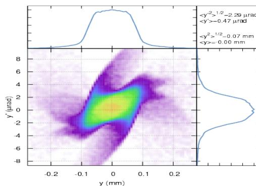
Figure 8: Vert. PS: 100 pC upstream FLASH2 undulator.
