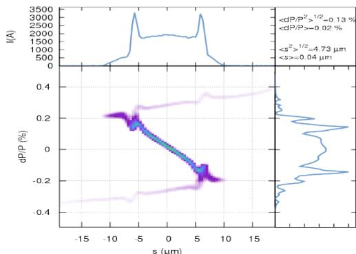
Figure 6: Long. PS: 100 pC upstream FLASH1 undulator.
