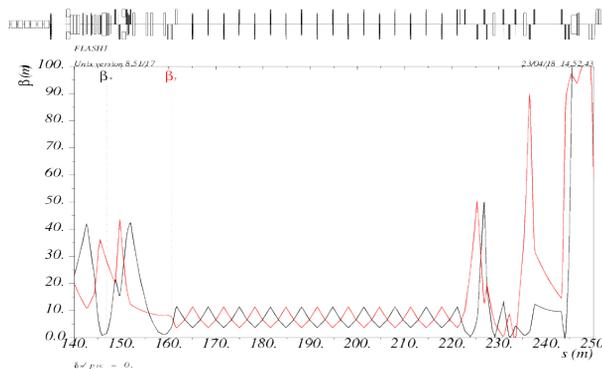
Figure 3: The upgraded optics in the FLASH1.
