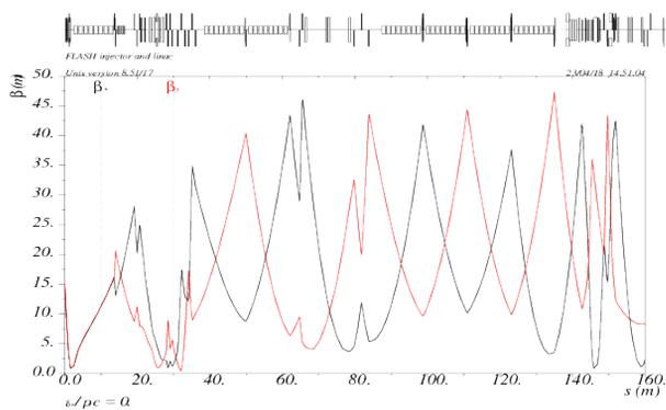
Figure 2: The upgraded optics in the FLASH injector & linac.
