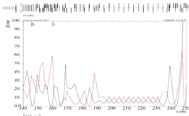
Figure 4: The upgraded optics in the FLASH2.
