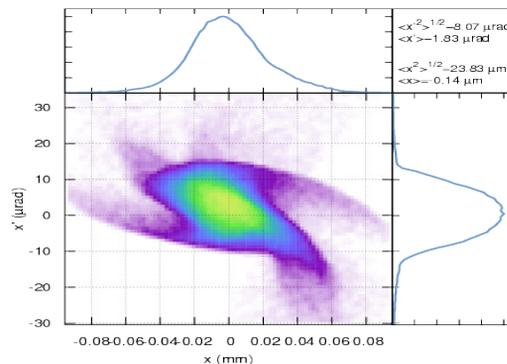
Figure 7: Hor. PS: 100 pC upstream FLASH2 undulator.
