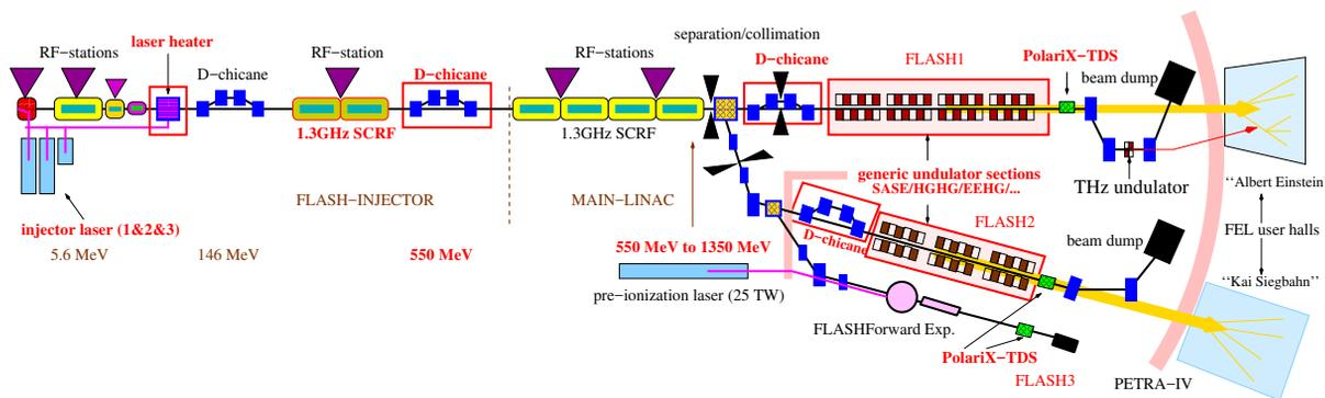
Figure 1: A possible scheme for the upgraded FLASH facility. Upgrade ideas are marked in red. Changes of the focusing lattice and changes of the beam optics are *not* indicated.
